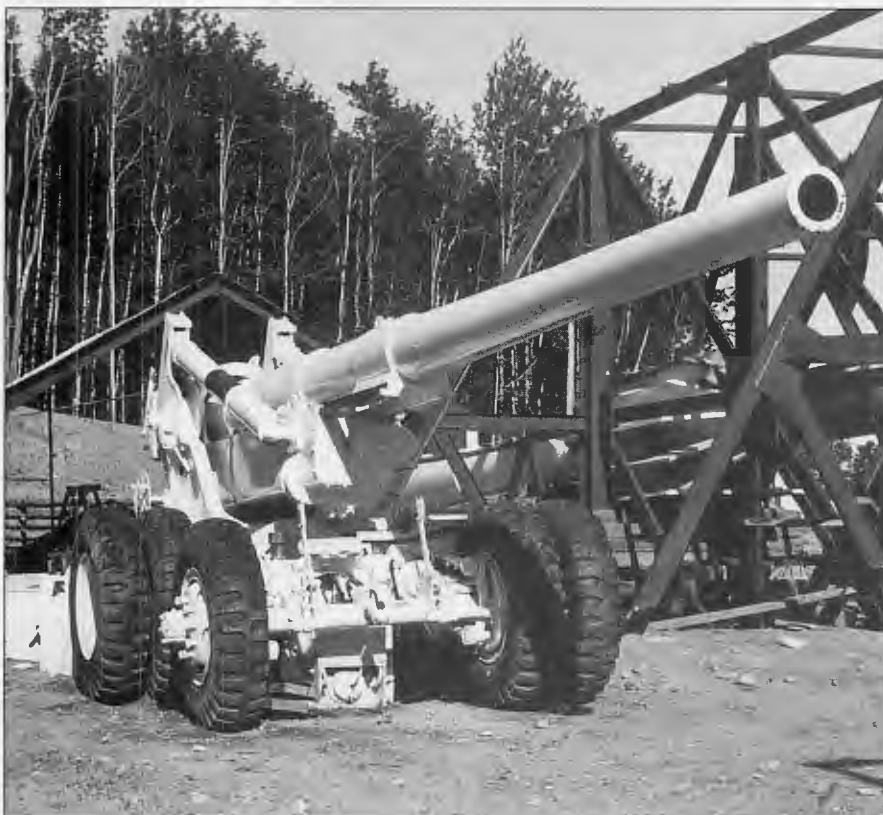
Sophisticated base-bleed and other advanced artillery technologies developed by Bull, such as for this 155mm prototype apparently based on a NORICUM gun, proved to be of wide interest: After having worked with U.S. Army, Bull was convicted of exporting technology to then-embargoed South Africa.
